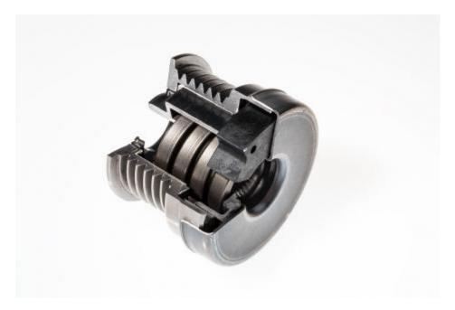
Our Decoupling Alternator Pulley (DAP) used with our Stretchy Belt to transfer power from the engine to parts in the front-end of the transmission. Thanks to our solution, you can now remove one or more idlers as well as the automatic tensioner, streamlining the front-end of the transmission.
