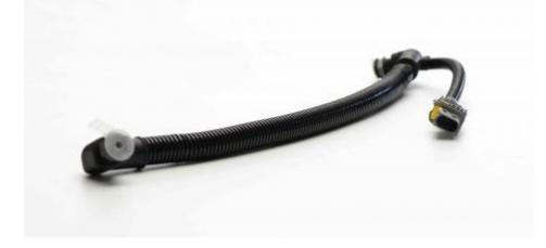
Our heated SCR line links the tank to the injection system on the exhaust line, supplying it with AdBlue® fluid. Our solution, created exclusively with thermoset thermoplastic materials, is lightweight and easy to install. Its heating power can be tailored to each customer's needs thanks to the smart choice of integrated resistant wires in the line wall.
